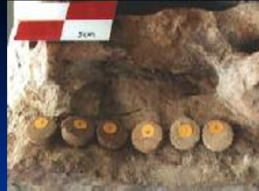
Colour-matched mortars for discreet repair
